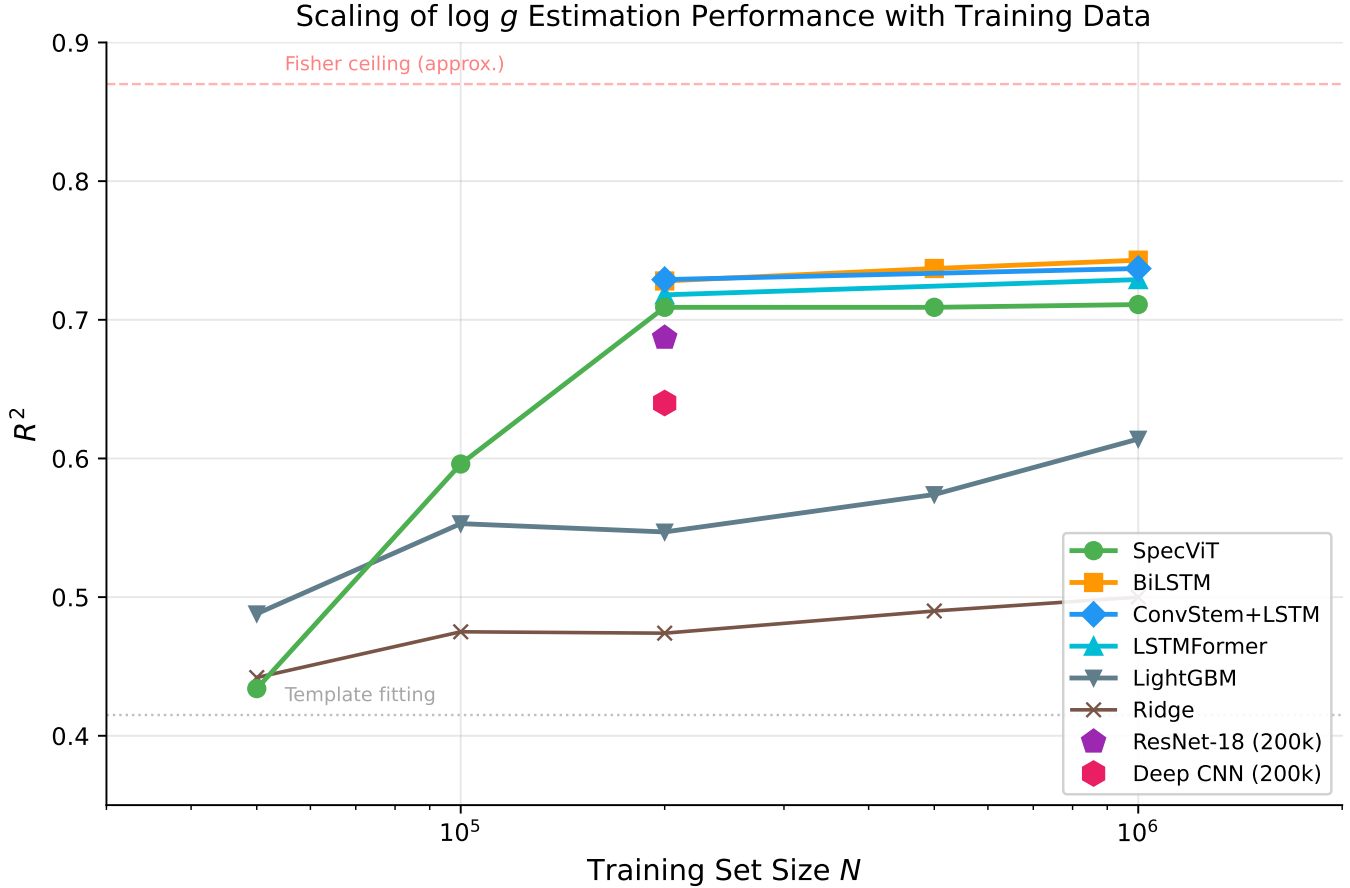
Figure 9. Scaling of test-set R^2 with training set size N for all architecture families. Deep learning models (solid lines) scale substantially more steeply than classical methods (dashed). At N = 2 \times 10^5 , BiLSTM and CONVSTEM+LSTM lead; the gap persists at N = 10^6 . The horizontal dashed line shows the Fisher information ceiling at \text{SNR} \approx 4.6 . All deep learning models saturate beyond N \gtrsim 5 \times 10^5 , likely reflecting the \sim 15,000 unique physical templates in the BOSZ grid rather than model capacity limitations.
